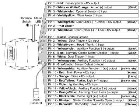
\*for positive (+12v) polarity locking and unlocking max current is 150mA
